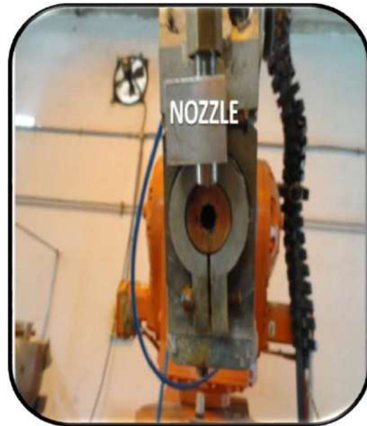
Plasma Gun Nozzle with Liquid Precursor or Powder Spray Deposition (2 – 5 \mu\text{m} / layer)
