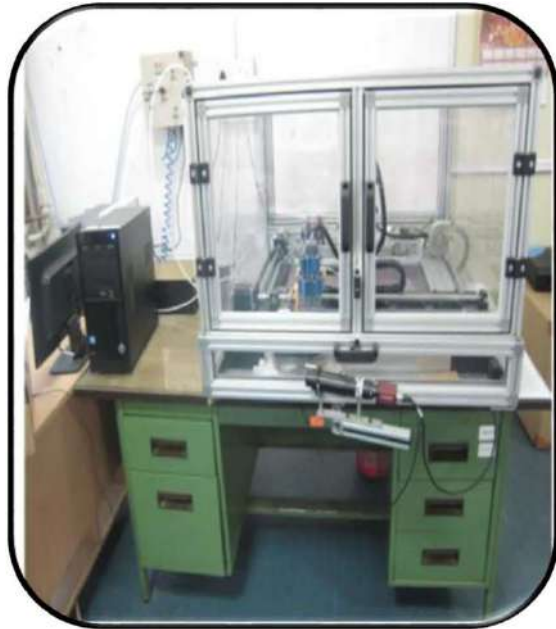
Ink Jet Printer - 16 nozzle assembly (Deposition : 0.5 \mu\text{m} / layer)
