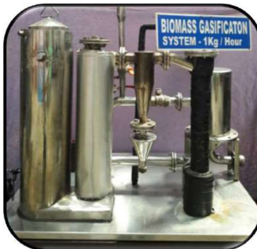
1 kW Biomass Gasification System
